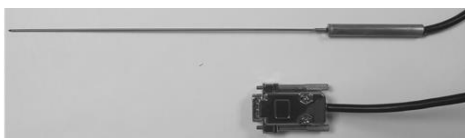
Fig. 2. Dosimetric needle with preamplifier and serial port connection.
