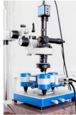
Fig. 1. AFM Scanning probe microscopy system JPK NanoWizard ® 3 [14]
