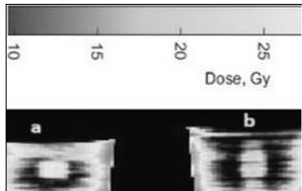
Fig. 9. Dose mapping of gels irradiated in a static mode (a) and in a rotating field (b).
