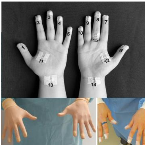
Fig. 2. Placement of the NaCl pellets (dosimeters) on the staff hands.
